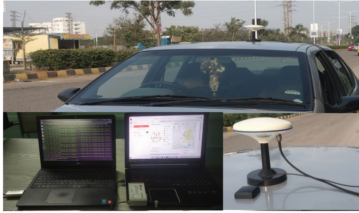
FIGURE 25 Experimental setup in dynamic case: with GNSS-SDR on the host PC, RTL-SDR and GNSS antenna for real-time processing of IRNSS/NavIC L5 signals, and a u-blox EVK-M8U receiver with antenna for reference
