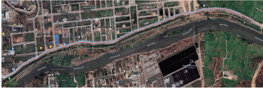
FIGURE 31 Google Maps show geodetic location coordinates obtained using GNSS-SDR in a dynamic case for IRNSS/NavIC L5 signals: The blue color trajectory is obtained with GNSS-SDR and the red color trajectory is the reference path obtained using a u-blox EVK-M8U hardware receiver
