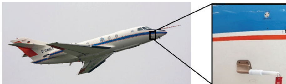
FIGURE 5 DLR's Dassault Falcon 20–E5, with an enlarged view of a static pressure port and Pitot tube on each of the two fuselage sides
