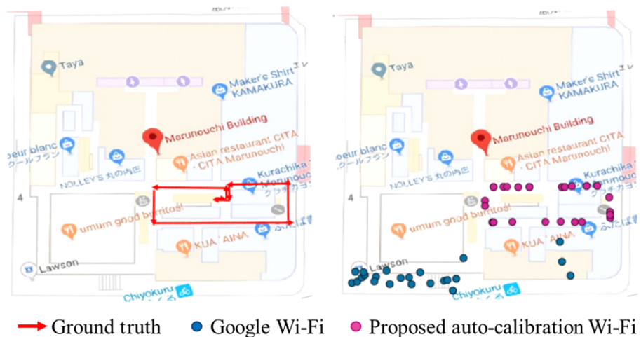
FIGURE 13 Ground truth of walking in test and Wi-Fi positioning results [Color figure can be viewed at wileyonlinelibrary.com and www.ion.org]
