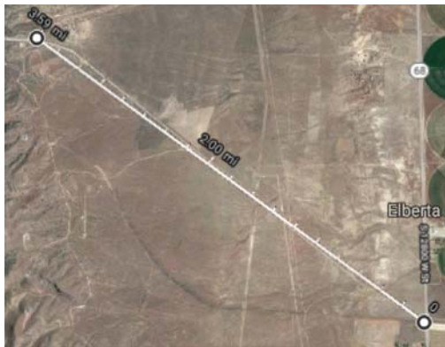
FIGURE 9 Left: The aircraft flight path during a manually flown flight test. Right: The true path is compared to the accumulated estimate. The estimates from 150 to 350 s are also shown to compare the result of removing most of the effects of the initialization errors. Other than the take-off and landing circles, the aircraft was flown approximately straight and level over a 6 km distance. Notice the scale bias in the estimates [Color figure can be viewed at wileyonlinelibrary.com and www.ion.org]
