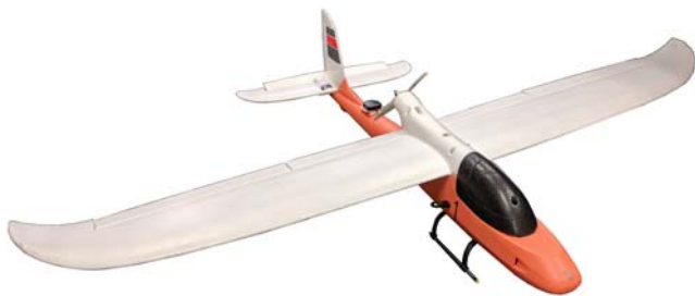
FIGURE 1 This work enables GPS-denied flight of fixed-wing UAS. The method was tested on a modified STRIX StratoSurfer, a 1.5 m wingspan aircraft [Color figure can be viewed at wileyonlinelibrary.com and www.ion.org ]
