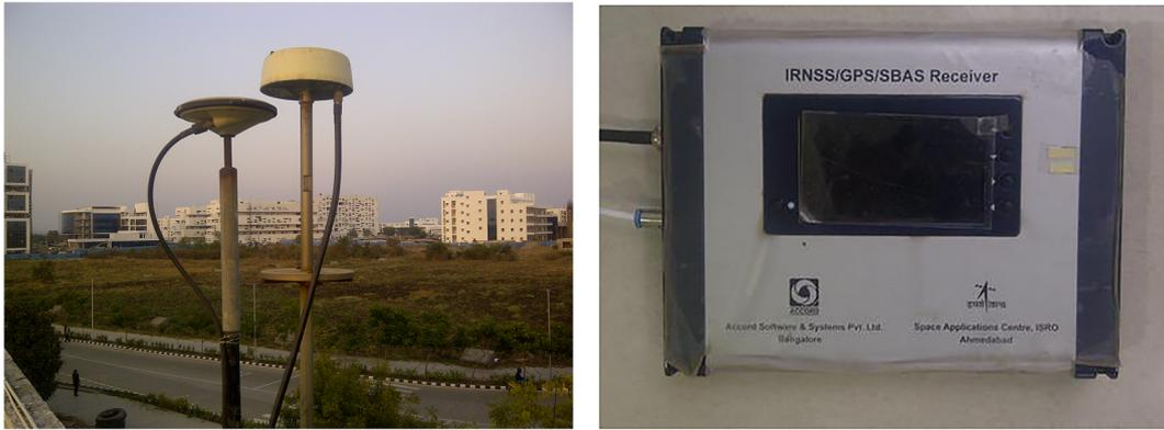
**FIGURE 1** (First plot) Accord's GNSS antenna (one on the right) in the Workshop building; (second plot) Accord's NavIC dual-frequency/GPS receiver [Color figure can be viewed at [wileyonlinelibrary.com](http://wileyonlinelibrary.com) and [www.ion.org](http://www.ion.org)]
