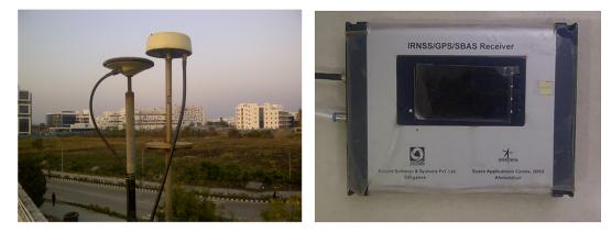
**FIGURE 1** (First plot) Accord's GNSS antenna (one on the right) in the Workshop building; (second plot) Accord's NavIC dual-frequency/GPS receiver [Color figure can be viewed at wileyonlinelibrary.com and www.ion.org]
