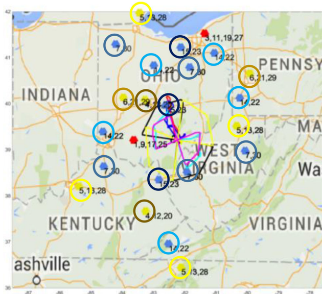
FIGURE 18 Test flight paths and ADS-B RS decoded (with assigned slot numbers indicated); ADS-B RS sharing the same slots are circled with the same shade of color [Color figure can be viewed in the online issue, which is available at wileyonlinelibrary.com and www.ion.org]
