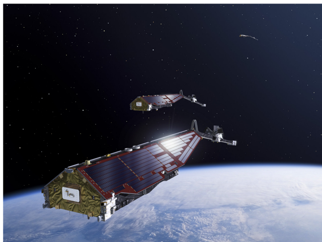
FIGURE 2 Artist's impression of the three original Swarm satellites. The booms point in the anti-flight direction. The two GPS antennas are mounted on the top side and nominally point towards zenith (image: ESA-P.Carril) [Color figure can be viewed in the online issue, which is available at wileyonlinelibrary.com and www.ion.org ]
