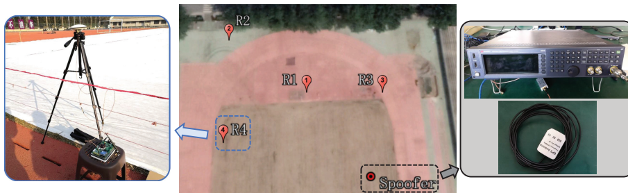
FIGURE 11 Deployment of the GPS receivers in the field experiment
