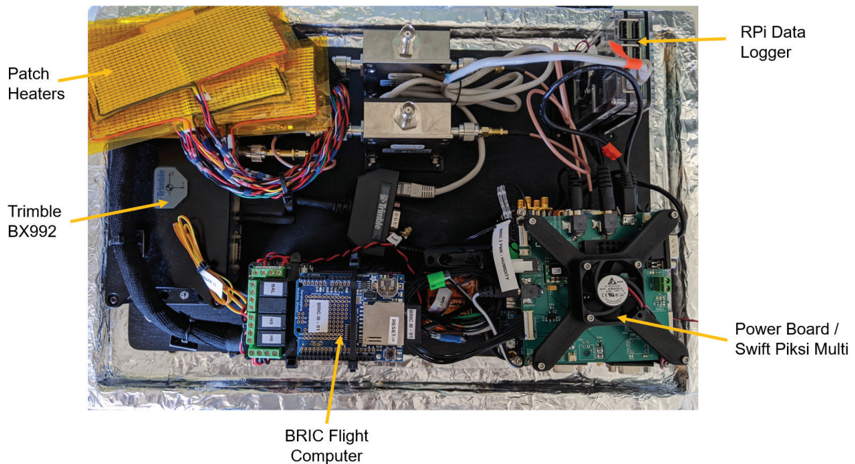
FIGURE 6 The GROOT system; a SwiftNav Piksi Multi recorded RO measurements, a Trimble BX992 generated precise position and velocity, and the data was logged to a RPi computer.
