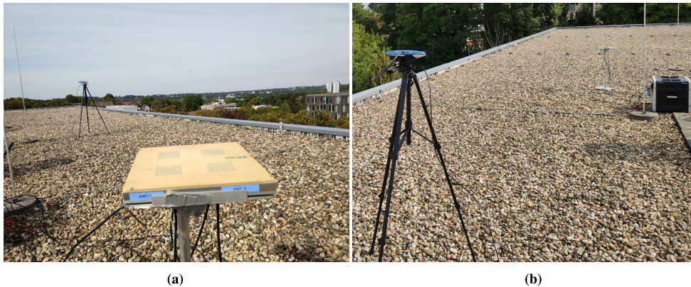
FIGURE 1 Measurement setup: The beige antenna array (DLR UNITAS) is used to receive the satellite signals, and the blue triangular-formed antenna is used to radiate the jamming signal.
