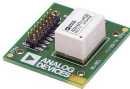
FIGURE 9 Analog Devices ADIS16470 MEMS IMU: The device footprint measures approximately 1.25'' \times 1.35'' .
