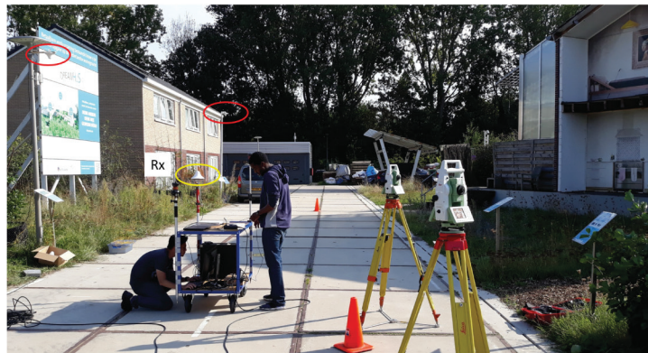
FIGURE 8 Prototype setup at The Green Village. Two of the transmitter antennas are visible in the lamp posts to the left (in red circles). The receiver antenna Rx (in yellow circle) is fixed to the trolley. The land-surveying stations at the right are used to provide the ground-truth trajectory of the receiver.
